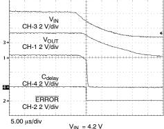
$\begin{array}{l} V_{IN} \; = \; 4.2 \; V \\ V_{OUT} \; = \; 3.3 \; V \\ C_{delay} \; = \; 0.1 \; \mu F \\ C_{NOISE} \; = \; 0.1 \; \mu F \\ I_{LOAD} \; = \; 350 \; mA \end{array}$
